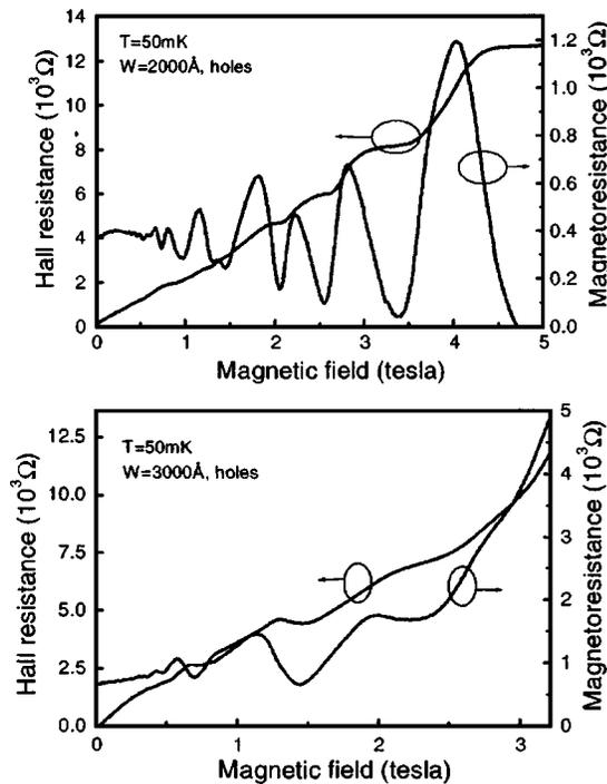
FIG. 2. Magnetoresistance (right axis) and Hall resistance (left axis) measurements carried out at 50 mK in the *p*-type samples containing a 2000-Å-wide (top) and 3000-Å-wide (bottom) PQW. The Hall bar was oriented along the  $[2\bar{3}3]$  direction and the magnetic field was applied perpendicularly to the sample.
