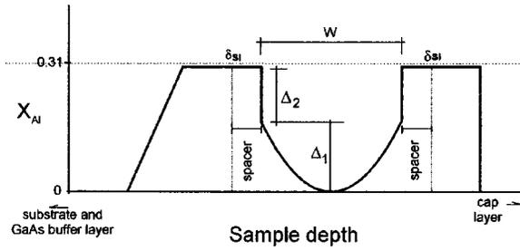
FIG. 1. Al composition ( $X_{Al}$ ) profile of our samples along the growth direction.  $W$  is the well width,  $\Delta_1$  is the maximum Al content of the parabolic profile, and  $\Delta_2$  was used to increase the barrier height and is equal to 0.11 for the 1000-Å-thick PQW and to 0.04 for the other two samples.
